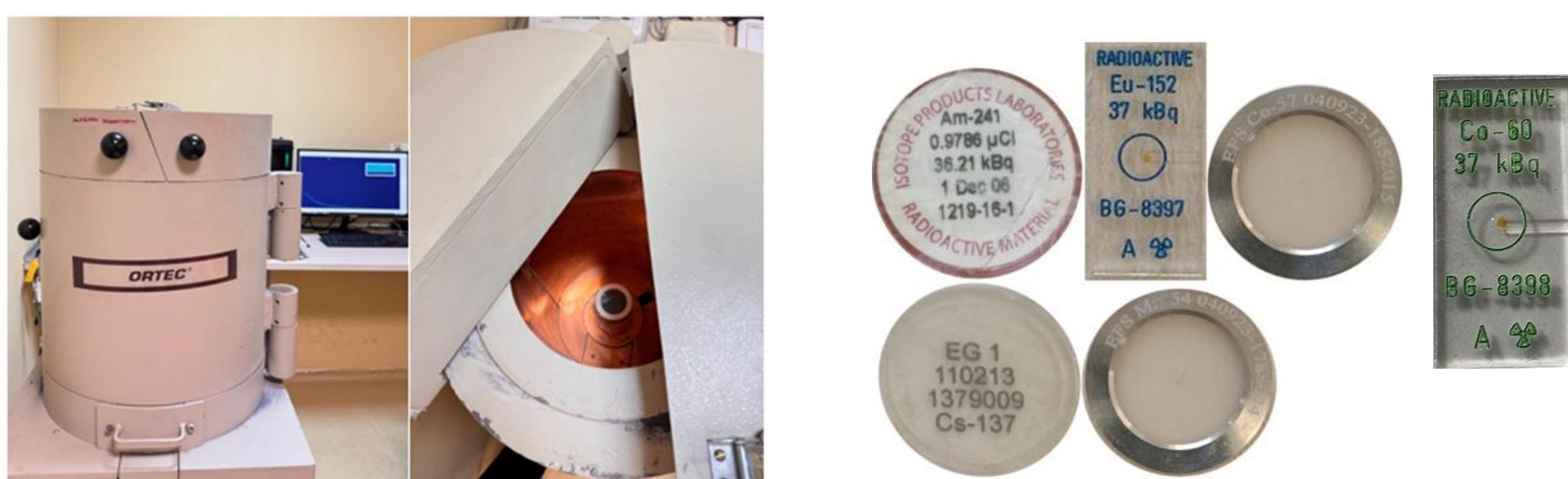
Figure 1. The HPGe detector and radioactive point sources used in the measurements.
