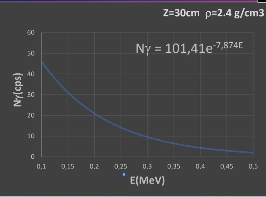
Energy spectra of the recorded  $\gamma$  in the energy bin [0.1 MeV, 0.5 MeV] at a distance of Z=30 cm from the neutron generator and for different densities
