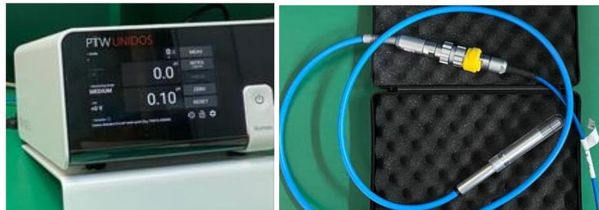
Electrometer + ionization chamber
