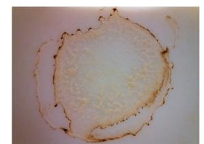
Figure 3. The reddish-white compound that remained after the purification of the white solid fragments from the mortar, similar to perlite
