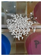
Figure 2. Separated white granules after physico-chemical pre-treatments
