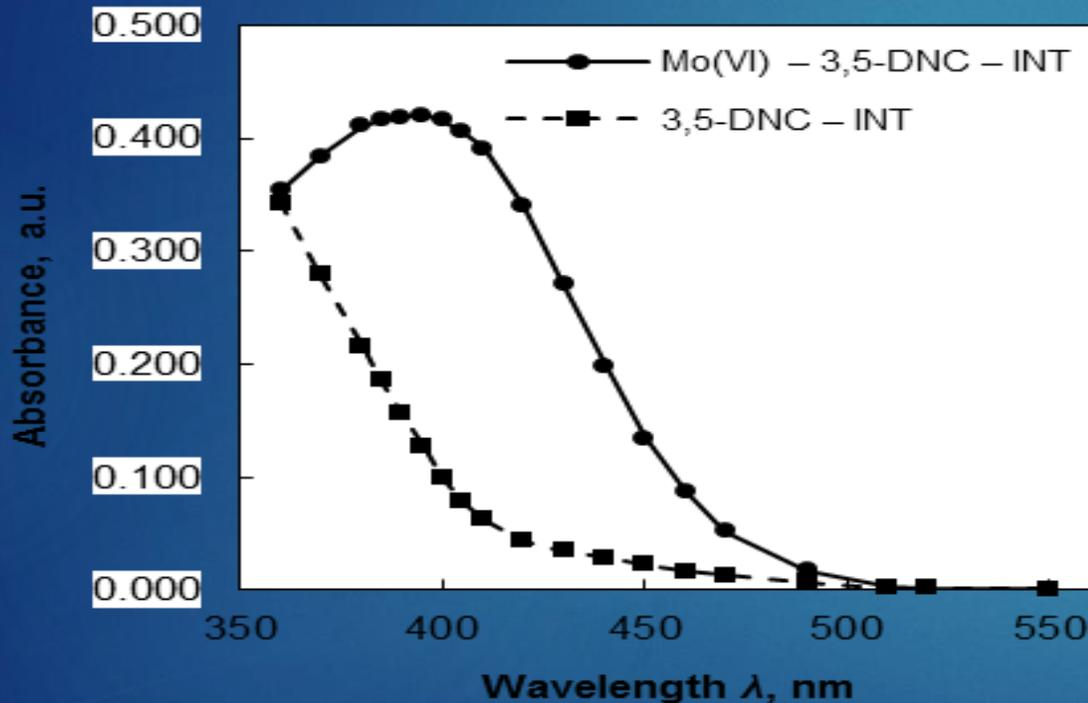
**Figure 1.** Absorption spectra of the complex Mo(VI)–3,5-DNC–INT and of the blank sample 3,5-DNC–INT in  $\text{CHCl}_3$
